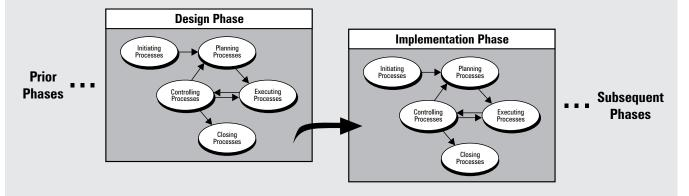
Although Figure 3–3 is drawn with discrete phases and discrete processes, in an actual project there will be many overlaps. The planning process, for example, must not only provide details of the work to be done to bring the current phase of the project to successful completion but must also provide some preliminary description of work to be done in later phases. This progressive detailing of the project plan is often called *rolling wave planning*.
